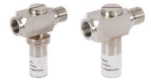
Made to safeguard pressure gauges and circuit pressure switches where high overpressures can be generated. Either by accidental causes the pressure exceeds the maximum value allowed, the limiter automatically exits the circuit to the instrument and automatically re-enters it when the process pressure returns to normal. The operating pressure is controllable over a wide range.
