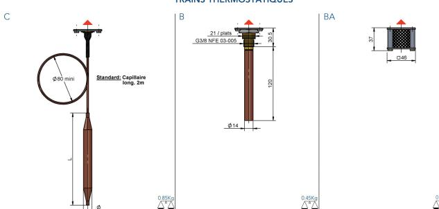
The triangles ▲ (shown on front view) and △ (shown on right-hand view) represent the assembled instrument. 2D or 3D drawings are available as an option to be specified in the order.
