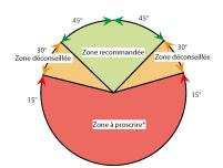
Recommended area: ±45° either side of the vertical axis, bulb down (capillary output up).
