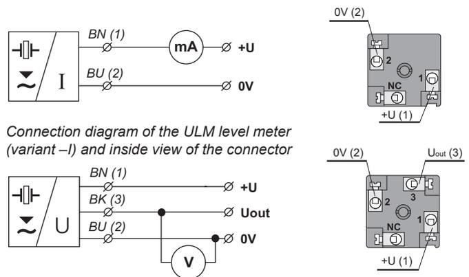
Connection diagram of the ULM level meter (variant -I) and inside view of the connector
