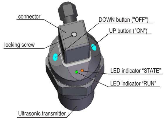
Key parts of the measuring device
