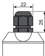
**Variant "H" with outlet for protective conductor**
