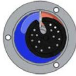
3- The liquid fills the inlet measuring chamber progressively (in red), as it is getting emptied on the outlet (in blue). In the middle of the cycle (see figure) the two chambers are the same size.
