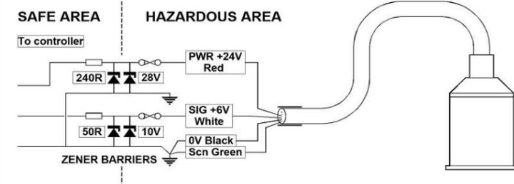
**Ex mb version:** This model must be supplied from apparatus that provides protection from prospective short circuits  $\geq 1500A$ .
