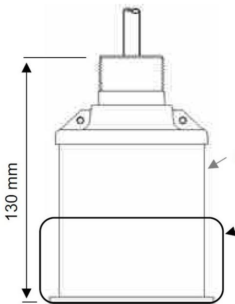
Radar Drawing with Drip Shield
