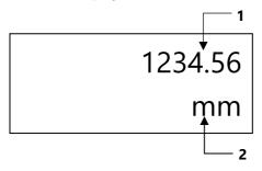
2) Auxiliary Display, scrolling 12-digit alpha numeric display Run Mode: displays units, totaliser or status messages on communications, detail of Hot Key function selected. Program Mode: displays Menu and Sub Menu headings, parameter details and options.
