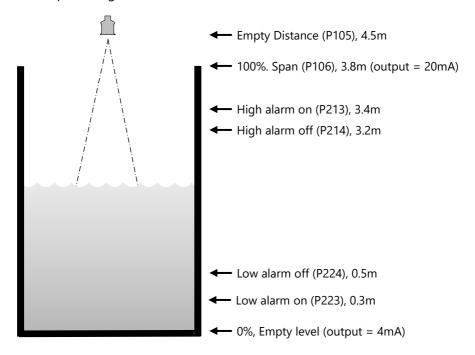
In this example, if the level rises to 3.4 m, then the high-level alarm (relay 1) will come on until the level drops to 3.2 m. If the level falls to 0.3m, then the low-level alarm (relay 2) will come on until the level rises to 0.5 m.
