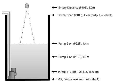
In this example a BlackBox with dB6 is being used to control pumps on a **pump down** application, there are two pumps, and the **duty** pump is to be **alternated** between the pumps.
