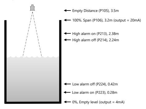
In this example, the BlackBox and dB6 is being used to monitor a moving level within a vessel and is required to provide a 4 to 20mA output proportional to the level, over a range of 3.2m. In addition to when the level rises to 2.5m, Relay '1' is required to give a high alarm and rest when the level falls to 2.4m. If the level should fall to 0.5m then Relay '2' is to give a low alarm and reset once the level rise to 0.6m.
