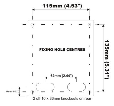
The BlackBox should be mounted by drilling four holes suitable for size 8 screws (length and type to suit your application) And fix all four screws by removing the top cover to access the pre-moulded mounting holes which are in the base of the enclosure under the lid retaining screws
