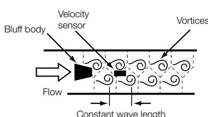
The measuring principle is based on the Kármán vortex street. A specially shaped bluff body is located in direction of the flow. From a certain flow velocity on vortices are generated through the bluff body.
