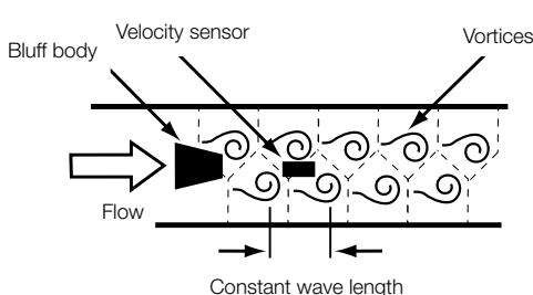
The measuring principle is based on the Karman vortex street. A specially shaped bluff body is located in direction of the flow. From a certain flow velocity on vortices are generated through the bluff body.
