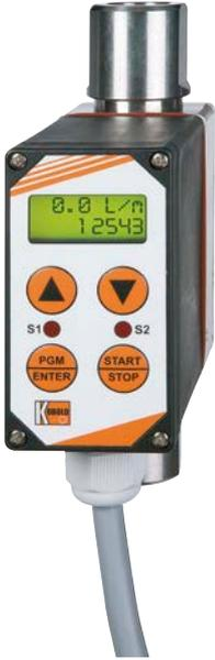
The evaluation unit changes the frequency signal of the pickup into a 3(4)-digit flow reading with adjustable scale (top line of display), and a scalable analogue signal. The dosage is displayed in the bottom line of the display. The unit of measurement can be selected. Included are two relays with floated output changeover contacts for various functions. The relay (S1) can be used to execute the flow monitoring, total volume monitoring, fine dosage or the pump control.
