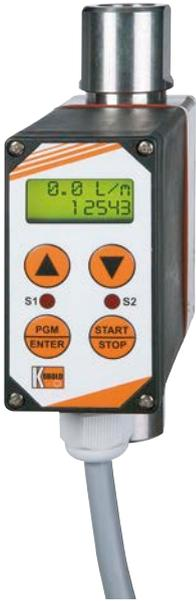
The evaluation unit changes the frequency signal of the pickup into a 3(4)-digit flow reading with selectable measurement unit (top display line), and into a scalable analogue signal. The flow quantity is added up in a part quantity meter and a total quantity meter and then displayed in the bottom line of the screen. The quantity meter's units of measurement are selectable.
