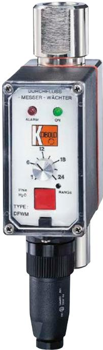
The DF-...WM evaluating electronics is used in applications where sporadic flow rate measurement is required, or where simultaneous continuous monitoring is needed. It converts the digital frequency signal from the sensor to a limit contact.
