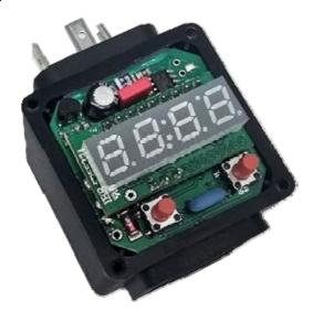
When turning, make sure that the rubber disk glued to the back of the electronic module does not fall out or get caught. Furthermore, make sure that when repositioning the electronic module, the supply wires remain behind the rubber disk and do not slip between the rubber disk and the electronic circuit board.
