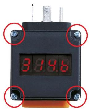
and the lid is carefully removed (so as not to damage any glued lid seal).
